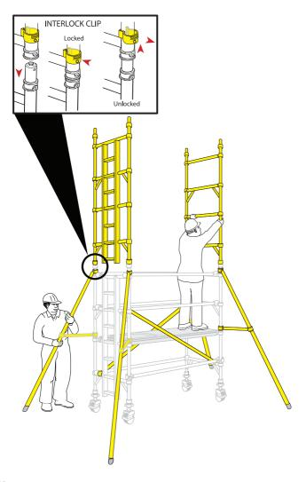
**4** Fit 2 pairs of diagonal braces in opposing directions between the 3rd and 5th rungs and the 5th and7th rungs. Locate a trapdoor deck on the 6th rung, with the trapdoor next to the ladder.
