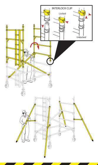
**5** Fit a temporary deck on the lowest rungs. Fit a trapdoor deck on the 4th rung (2.0m) with the trapdoor next to the ladder. Ensure the trapdoor is positioned with the hinges towards the outside of the tower as shown. Climb the ladder and, from the protected trapdoor position, fit guardrails on the 5th and 6th rungs (in that order) on both sides of the platform.
