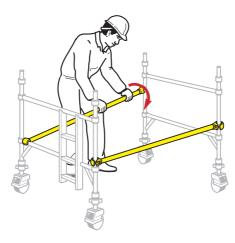
Fit 2 additional end frames ensuring the frame interlock clips are engaged. Fit 2 diagonal braces (blue) in opposing directions, between the 1st and the 3rd rungs. Ensure the frames are vertical and level by checking with a spirit level and setting the adjustable legs as required. Fit stabilisers **(see noteson page 30)**.
