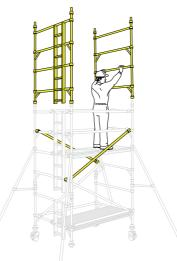
Add two more diagonal braces between the 5th and 7th rungs. If finishing at this height (4.2m platform), reposition the fixed deck to the 8th rung on the tower. Fit a trapdoor deck alongside it, with the hinges towards the outside of the tower, and the trapdoor next to the ladder. Add a single diagonal between the 7th and 9th rungs as shown. Climb up the ladder, and from the protected trapdoor position, fit the guardrails on the 9th and 10th rungs, in that order, on both sides of the tower.
