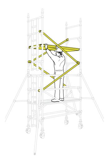
**5** Climb up the inside of the tower and from the protected position of the trapdoor, fit guardrails to the 7th and 8th rungs, (in that order), on both sides of the tower.
