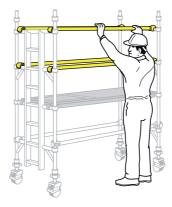
**3** Fit 2 diagonal braces in opposing directions between the 1st and 3rd rungs. Ensure the frames are vertical and level by checking with a spirit level and setting the adjustable legs as necessary. Fit stabilisers (see notes on **page 30**). Fit the next pair of end frames and check the frame interlock clips are engaged.
