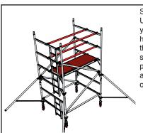
Step 6. Using the 3T method, position yourself in the hatch and fit four horizontal guardrail braces on the fifth and sixth rungs to either side of the platform. Access the platform and secure the braces and diagonal brace at the opposite end of the tower.
