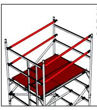
Step.9 Using the 3T method install 4 horizontal guardrail braces onto ninth and tenth rungs to both sides of the tower.
