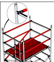
Step.10 Access the platform and secure the horizontal guardrail braces and last diagonal brace at the opposite end of the tower.
