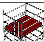
Step 11. Fit the toeboard set ensuring the edges of the toeboard overlap the platform edges on all four edges
