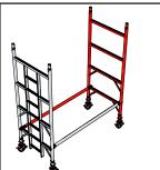
Step 3. Join the second 4 rung frame to the first ensuring that the brace hook is resting on the opposite horizontal rung. Fit the second brace to the horizontal tubes as shown with hook apertures facing downwards. Level around base of tower using spirit level, making adjustments as necessary to adjustable legs until the frames have an inclination no more than 1% from the vertical.
