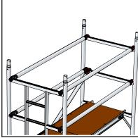
Access the platform and secure the horizontal guardrail braces and last diagonal brace at the opposite end of the tower.
