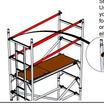
Step.9 Using the 3T method, position yourself in the hatch and install four horizontal guardrail braces onto seventh and eigth rungs to either side of the platform.
