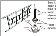
Insert castor/adjustable leg assemblies into base of 4 rung ladder frame and one 4 rung frame, allowing approximately 75mm of extended leg for levelling.
